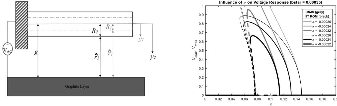
Figure 1: (Left) Electrostatically actuated DWCNT cantilever resonator. (Right) Effect of frequency on the amplitude-voltage response of parametric resonance of coaxial vibrations of electrostatically actuated DWCNT.
